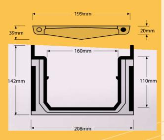
Simple jointing system – male and female joiners slide together to maintain alignment.
